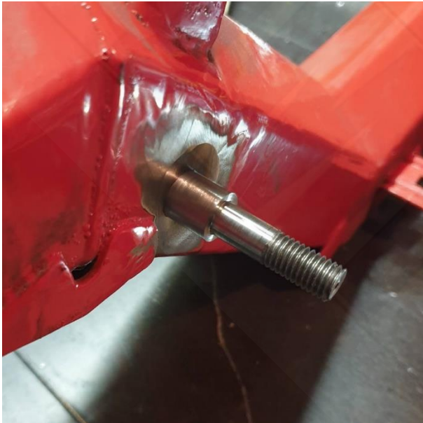
Image 5: Center the new shock absorber bolt
