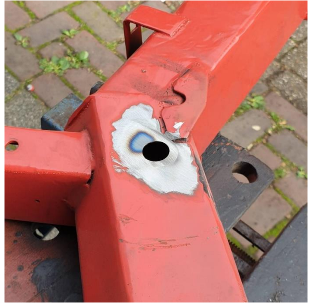
Image 4: Hole for the new shock absorber bolt
