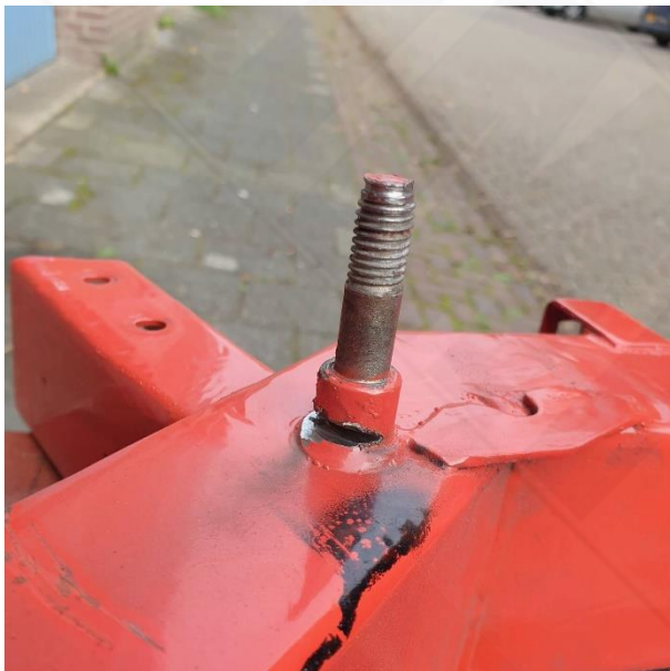
Image 2: Cut of the damaged bolts
